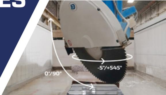
**Sliding cross-beams and bridge** with linear bearings and helicoidal-teeth racks for the X and Y axis, with lubrication by automated grease system and bellows for protection with labyrinth closure.
